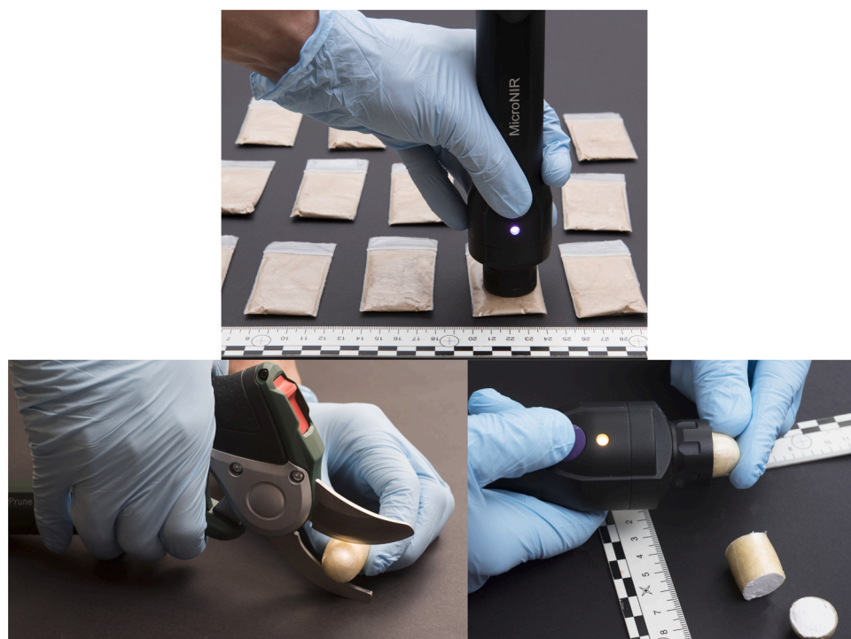
Fig. 2. Top: Measurements through the plastic of an heroin bag, Bottom left: Cutting a cocaine finger with an electric sheering prune, Bottom right: Measurements on the finger slices.
