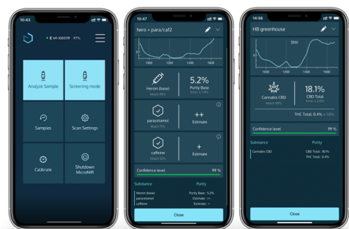
Figure 2 – NIRLAB mobile app screen, showing the results of a single scan.
