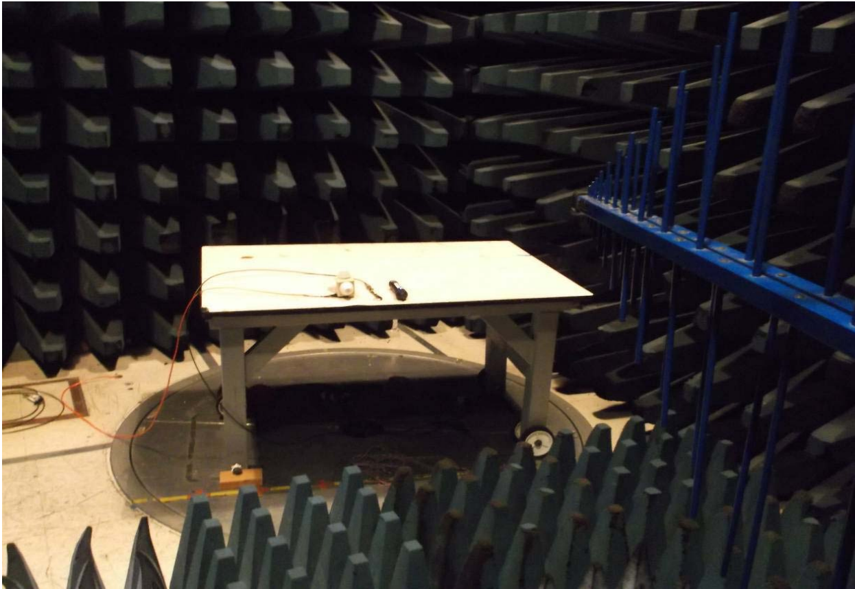
Test Configuration Photograph #1 (Radiated Immunity, EN 61000-4-3)
